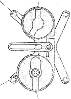
female airline fitting. Threaded hole is ¾" NPT.
